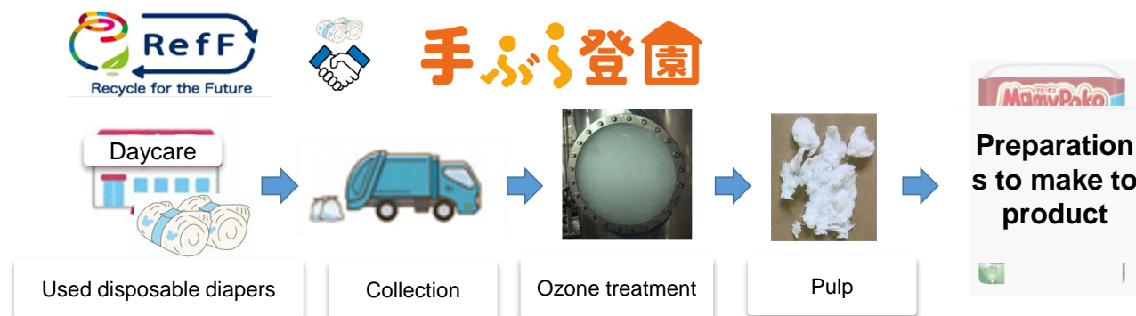
Process flow recycling from collecting used diapers from daycare facilities to creating new product
